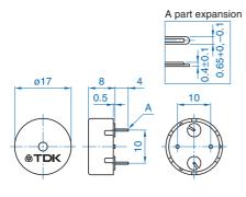
Tolerance: ±0.3 Dimensions in mm
