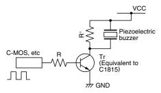
$^{\circ}$  Resistor to do charging and discharging to a piezoelectric element (Value of about 1k $\Omega$  is good efficiency).
