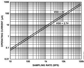
Figure 25. Operating Current vs. Sampling Rate
