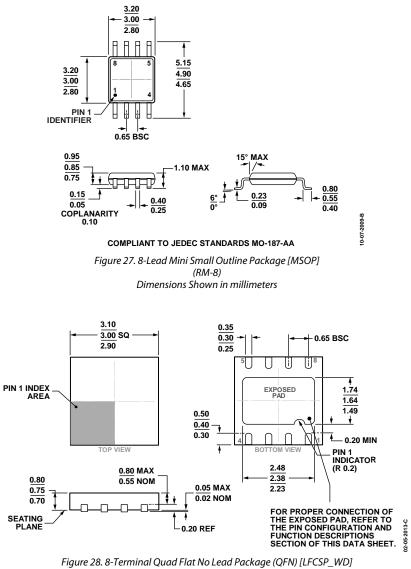
Figure 28. 8-Terminal Quad Flat No Lead Package (QFN) [LFCSP\_WD] 3 mm × 3 mm Body, Very Very Thin, Dual Lead (CP-8-3) Dimensions Shown in millimeters
