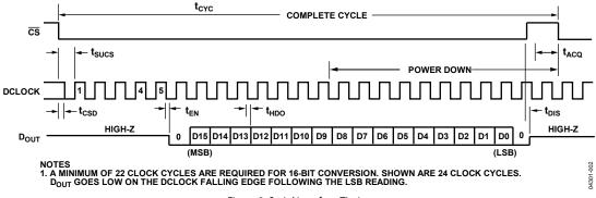
Figure 2. Serial Interface Timing
