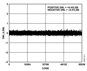
Figure 11. Differential Nonlinearity vs. Code
