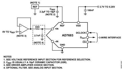
Figure 23. Typical Application Diagram
