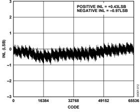
Figure 8. Integral Nonlinearity vs. Code
