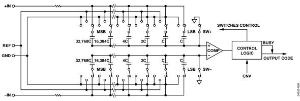
Figure 21. ADC Simplified Schematic
