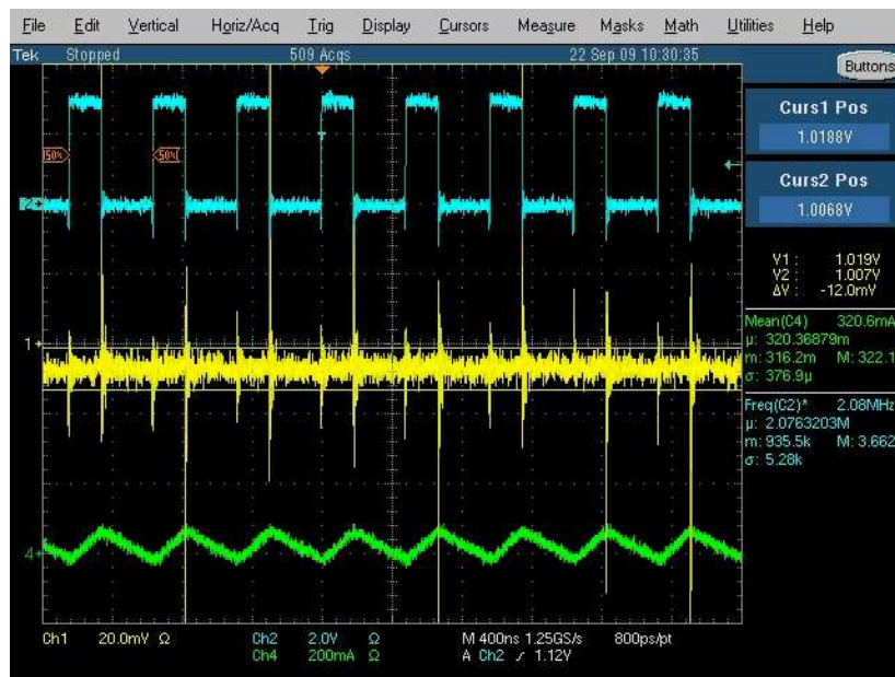
Figure 17. L=GLK2510P-4R7M, C=Ceramic 4.7 \mu F 0805 X5R TDK (Ripple 12mV)
