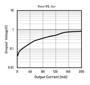
Fig4. Dropout Voltage VS Output Current
