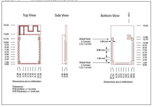
FIGURE 4-2: RN4020 RECOMMENDED PCB FOOTPRINT
