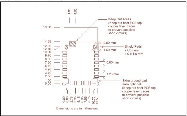
FIGURE 4-3: RN4020 MODULE MOUNTING DETAILS
