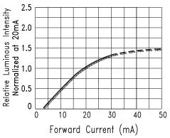
Fig.4 Relative Luminous Intensity vs. Forward Current
