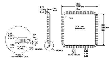
COMPLIANT TO JEDEC STANDARDS MS-026-BEC Figure 5. 80-Lead Low Profile Quad Flat Package [LQFP] (ST-80-2)
