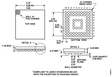
Figure 7. 76-Ball Chip Scale Package Ball Grid Array [CSP\_BGA] 6 mm × 6 mm × 1.4 mm (BC-76-1) Dimensions shown in millimeters
