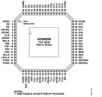
Figure 3. 64-Lead LFCSP Pin Configuration (Top View)
