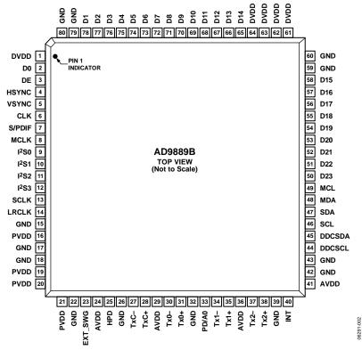
Figure 2. 80-Lead LQFP Pin Configuration (Top View)
