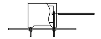
Temperature monitored inside the capacitor.
