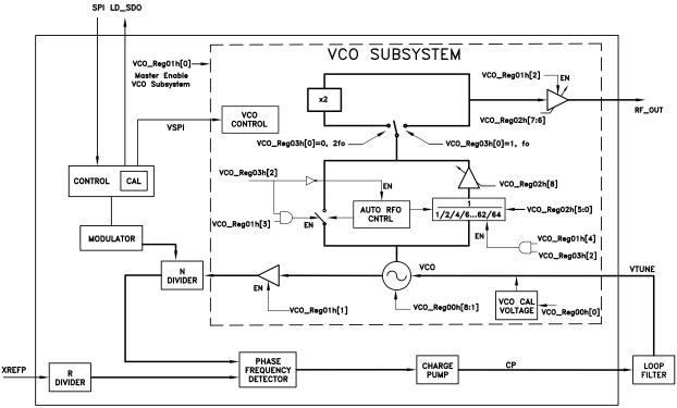
Figure 27. PLL and VCO Subsystems
