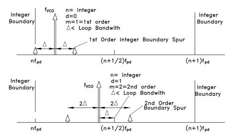
Figure 32. Fractional Spurious Example
