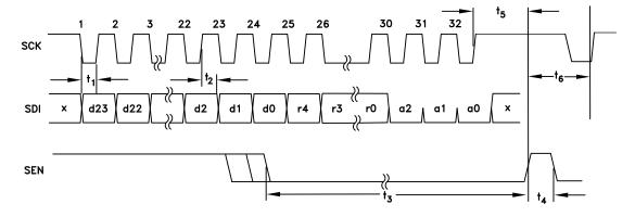
Figure 47. Open Mode - Serial Port Timing Diagram - WRITE
