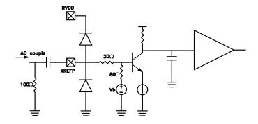
Figure 39. Reference Path Input Stage
