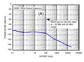
Figure 35. HMC833LP6GE Worst spur at any offset, fixed 50 MHz reference, output frequency = 2000.1 MHz
