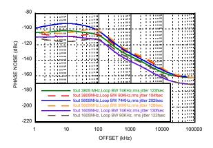
Figure 3. Free Running Phase Noise
