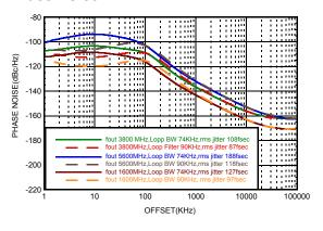
Figure 2. Typical Closed Loop Fractional Phase Noise<sup>[\*loop Filter Configuration Table\*]</sup>
