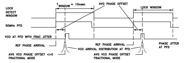
Figure 41. Lock Detect Window - Fractional Mode with Offset
