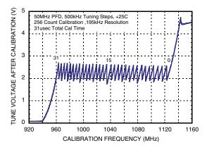
Figure 30. A Typical 5-Bit 32 Switch VCO Tuning Voltage After Calibration
