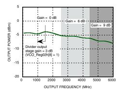
Figure 26. Reducing the output power variation of HMC833LP6GE across frequency by adjusting output stage gain control.
