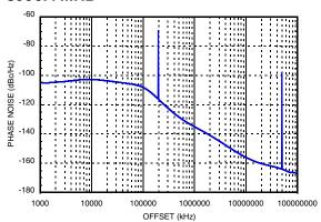
Figure 16. Fractional-N Exact Frequency Mode ON Performance at 2591 MHz<sup>[8]</sup>
