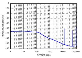
Figure 17. Fractional-N Exact Frequency Mode OFF Performance at 2591 MHz
