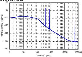
Figure 15. Fractional-N Exact Frequency Mode ON Performance at 2113.5 MHz<sup>[7]</sup>
