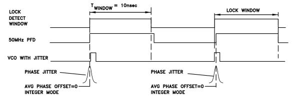
Figure 40. Normal Lock Detect Window - Integer Mode, Zero Offset
