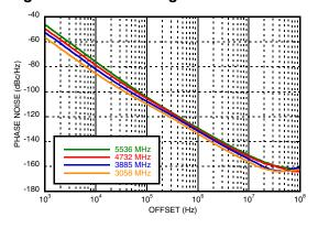
Figure 4. Free Running VCO Phase Noise vs. Temperature
