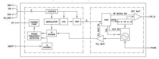
Figure 29. HMC833LP6GE PLL and VCO Subsystems
