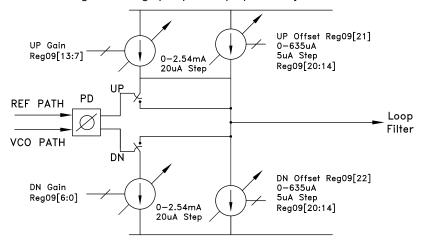
Figure 43. Charge Pump Gain & Offset Control
