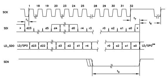
Figure 48. Serial Port Timing Diagram - READ
