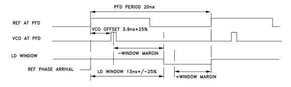
Figure 42. Lock Detect Window Example with 50 MHz PD and 3.9 ns VCO Offset
