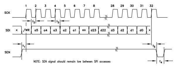
Figure 45. HMC Mode - Serial Port Timing Diagram - WRITE
