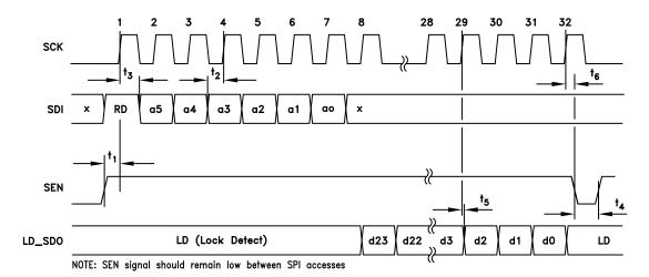
Figure 46. HMC Mode - Serial Port Timing Diagram - READ
