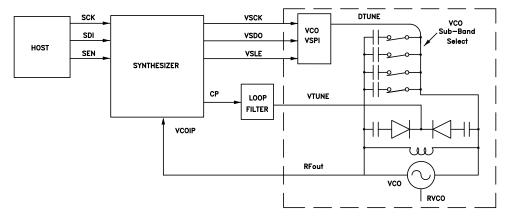
Figure 28. Simplified Step Tuned VCO
