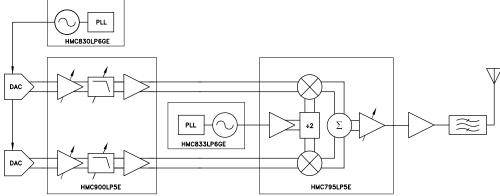
Figure 23. HMC833LP6GE in a typical transmit chain
