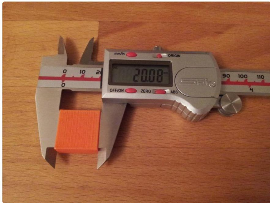
Scale calibration illustrates the process in which you compare the desired dimensions with the actual dimensions your printer produces. The easiest method for accomplishing this is to start by printing a calibration object, like a [Calibration Cube](https://adafru.it/cos) (<https://adafru.it/cos>) or the [Calibration Vector](https://adafru.it/cot) (<https://adafru.it/cot>). Once complete, use a set of calipers to check the dimensions and record your results.
