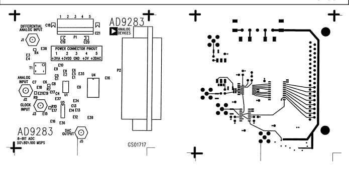
Figure 7. Printed Circuit Board Top Side Silkscreen
