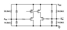
Figure 2. Equivalent Analog Input Circuit
