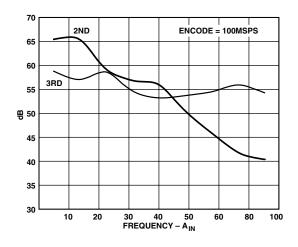
TPC 4. Harmonic Distortion vs. A<sub>IN</sub> Frequency
