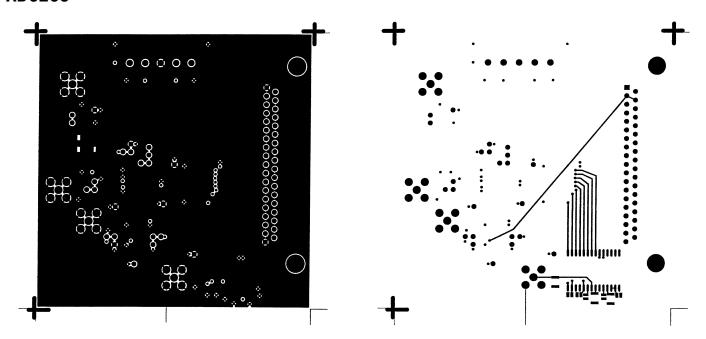
Figure 11. Printed Circuit Board Ground Layer
