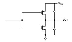
Figure 5. Equivalent Digital Output Circuit
