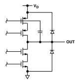
Figure 6. Equivalent Reference Output Circuit
