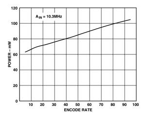
TPC 10. Analog Power Dissipation vs. Encode Rate
