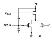
Figure 3. Equivalent Reference Input Circuit
