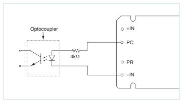
Figure 6 — Isolated on-state indicator
