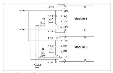
Figure 10 — Transformer-coupled interface
