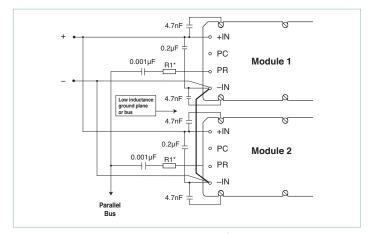
**Figure 9** — AC-coupled single-wire interface
