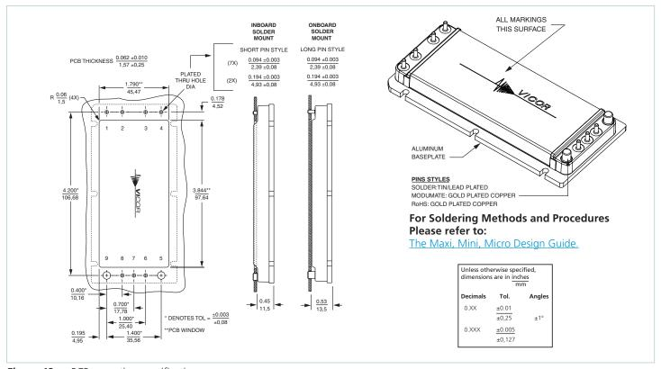
Figure 13 — PCB mounting specifications
