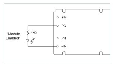
Figure 4 — LED on-state indicator
