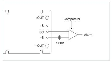
Figure 7 — Secondary side on-state indicator
