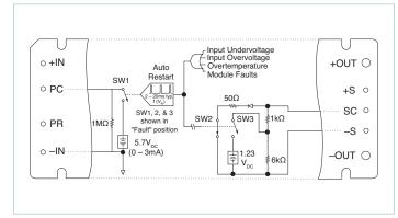
Figure 3 — PC/SC module alarm logic
