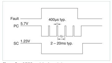
Figure 5 — PC/SC module alarm timing
