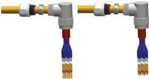
Step 7: Attach contacts to wire leads
