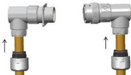
Step 11: Push shielding clip into backshell
