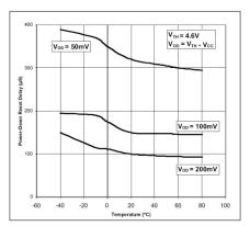
Fig. 7: Power-Down Reset Delay versus Temperature
