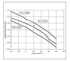
Fig. 8: Normalized Reset Threshold versus Temperature
