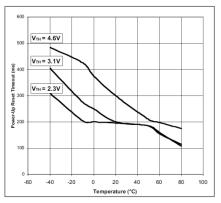
Fig. 9: Power-Up Reset Time-out versus Temperature
