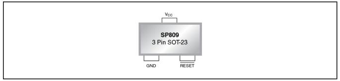
Fig. 3: SP809 Pin Assignment
