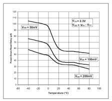
Fig. 5: Power-Down Reset Delay versus Temperature
