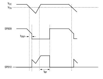
Fig. 10: Timing Waveforms
