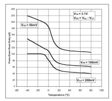
Fig. 6: Power-Down Reset Delay versus Temperature
