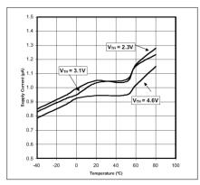
Fig. 4: Supply Current versus Temperature
