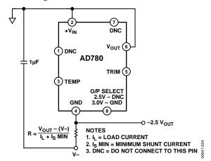
Figure 24. Negative (-2.5 V Shunt Mode Reference)
