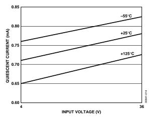
Figure 14. Typical Supply Current over Temperature
