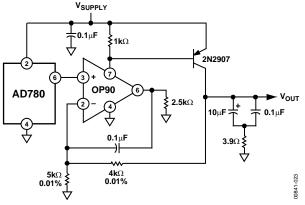
Figure 23. 4.5 V Reference from a Single 5 V Supply
