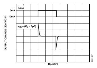
Figure 17. Settling Under Transient Resistive Load
