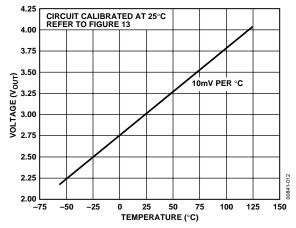
Figure 12. Temperature Pin Transfer Characteristic
