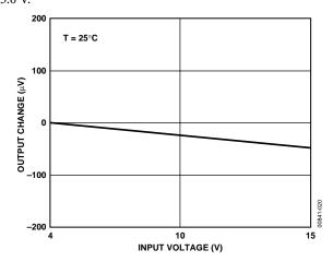
Figure 20. Output Voltage Change vs. Input Voltage
