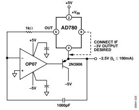
Figure 25. –2.5 V High Load Current Reference
