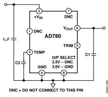
Figure 9. Noise Reduction Circuit
