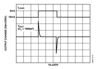
Figure 19. Settling under Dynamic Capacitive Load
