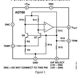
The AD780 is a pin compatible performance upgrade for the LT1019(A)–2.5 and the AD680. The latter is targeted toward low power applications.
