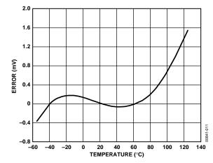
Figure 11. Typical AD780BN Temperature Drift
