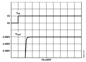
Figure 15. Turn-On Settling Time Performance
