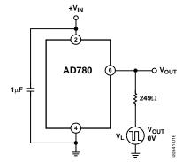
Figure 16. Transient Resistive Load Test Circuit
