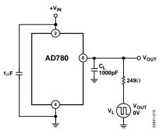
Figure 18. Capacitive Load Transient Response Test Circuit
