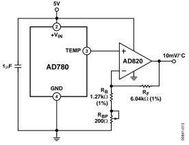
Figure 13. Differential Temperature Transducer
