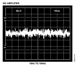
Figure 10. Reduced Noise Performance with  $C1 = 100 \mu F$ , C2 = 100 nF
