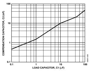
Figure 6. Compensation and Load Capacitor Combinations
