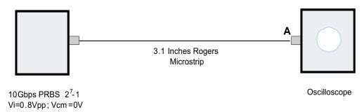
Figure 9. Source Eye Diagram Test Setup
