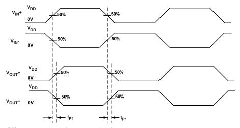
$T_{SKEWInter}$  = Difference between  $t_{PD}$  for any two pairs of outputs
