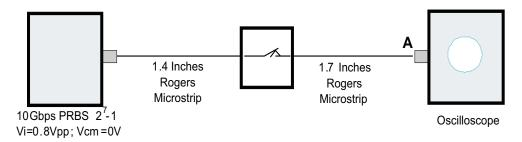
Figure 10. Output Eye Diagram Test Setup
