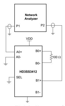
Figure 8. Off Isolation Measurement Setup
