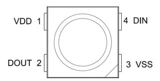
Figure 2. IN-PI55TAT(X)R(X)G(X)B Pin Configuration
