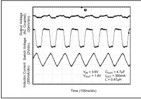
*FIGURE 2-19:* Switching Waveform - Continuous Mode.
