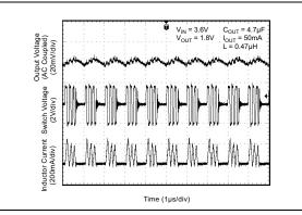
FIGURE 2-17: Switching Waveform - Discontinuous Mode.
