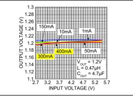
FIGURE 2-6: Output Voltage vs. Input Voltage.
