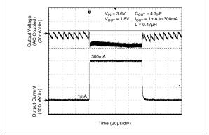
FIGURE 2-24: Load Transient.
