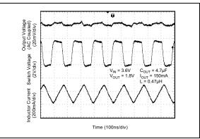
FIGURE 2-18: Switching Waveform - Continuous Mode.
