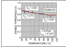
**FIGURE 2-13:** Enable Threshold vs. Temperature.
