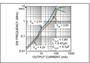
FIGURE 2-11: Switching Frequency vs. Output Current.
