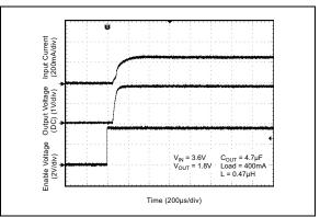
FIGURE 2-22: Start-Up Waveform.
