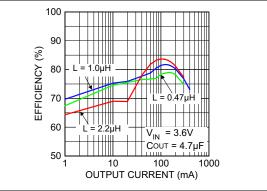
FIGURE 2-4: Efficiency with Various Inductors.
