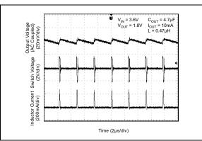
FIGURE 2-16: Switching Waveform - Discontinuous Mode.
