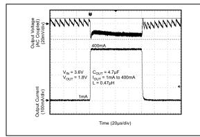
FIGURE 2-25: Load Transient.
