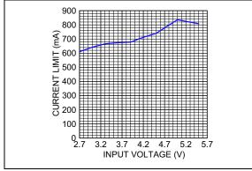
FIGURE 2-14: Current-Limit vs. Input Voltage.
