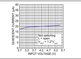
FIGURE 2-5: Quiescent Current vs. Input Voltage.
