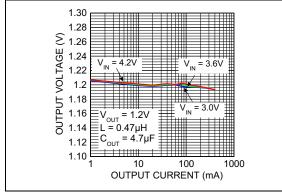
FIGURE 2-7: Output Voltage vs. Output Current.
