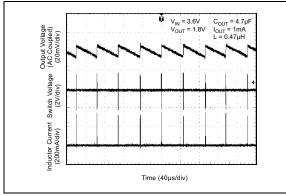
FIGURE 2-15: Switching Waveform - Discontinuous Mode.
