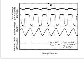
FIGURE 2-20: Switching Waveform - Continuous Mode.
