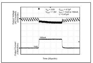
FIGURE 2-23: Load Transient.
