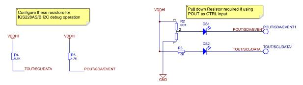
Figure 2.5: IQS228AS/B output pin configuration for I2C debug operation, or driving LEDs (active high or low option available).
