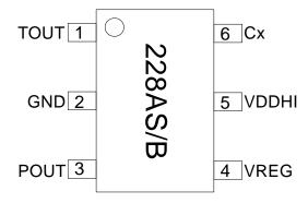
Figure 2.1:Pin-out of IQS228AS/B in the TSOT23-6 package.
