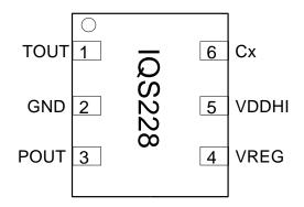
Figure 2.3: Pin-out of IQS228B in DFN-6 package.
