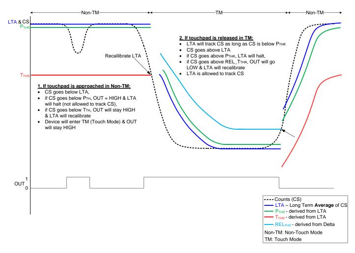
Figure 5.1: DYCAL Operation (Self Capacitive Sensing)
