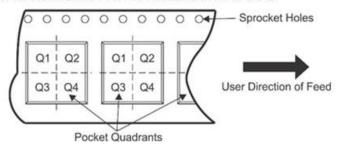
Figure 12.7: TSOT23-6 Tape Specification.
