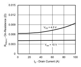
On-Resistance vs. Drain Current and Gate Voltage
