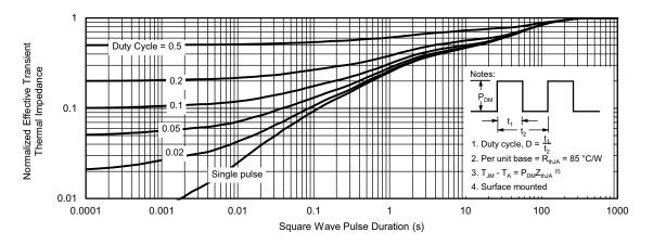
Normalized Thermal Transient Impedance, Junction-to-Ambient
