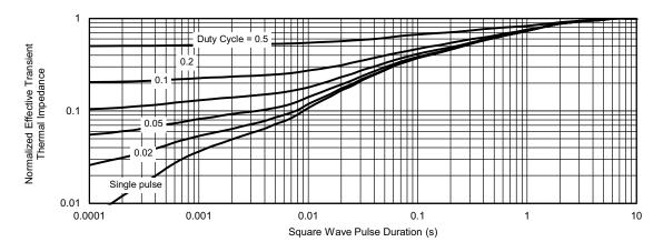
Normalized Thermal Transient Impedance, Junction-to-Case
