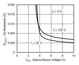
On-Resistance vs. Gate-to-Source Voltage
