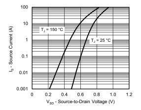
Source-Drain Diode Forward Voltage
