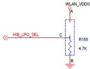
RF\_SW\_CTRL\_9 can also be used for LPO Selection. However, it should be pulled LOW to use the recommended external 32.768-kHz HIB crystal.
