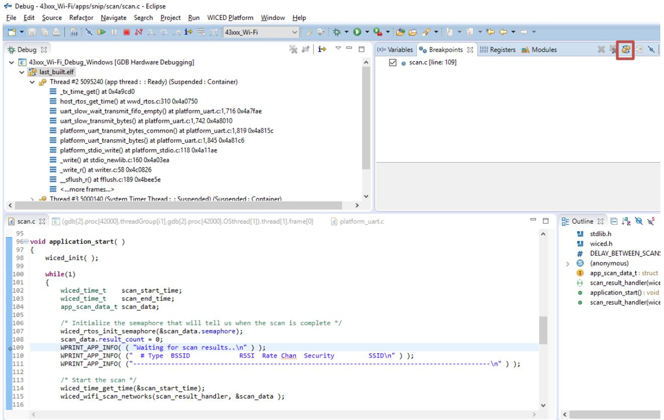
Figure 3-10. Enabling Breakpoint for Current Execution
