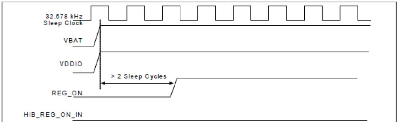
Figure 38. HIB\_REG\_ON\_IN = HIGH, HIB\_REG\_ON\_OUT Connected to REG\_ON
