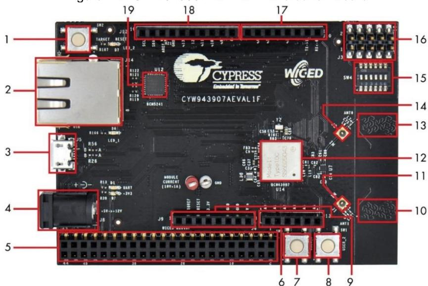
Figure 1-3. CYW943907AEVAL1F Evaluation Board (Back View)
