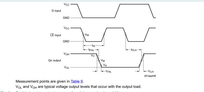
Fig. 8. Enable input to output propagation delays and pulse width
