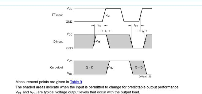
Fig. 10. Data input to latch enable input set-up and hold times
