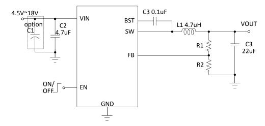
**Note:** The application scenario is that the DC power supply is directly plugged in, and it is recommended to add electrolytic capacitance at the input.
