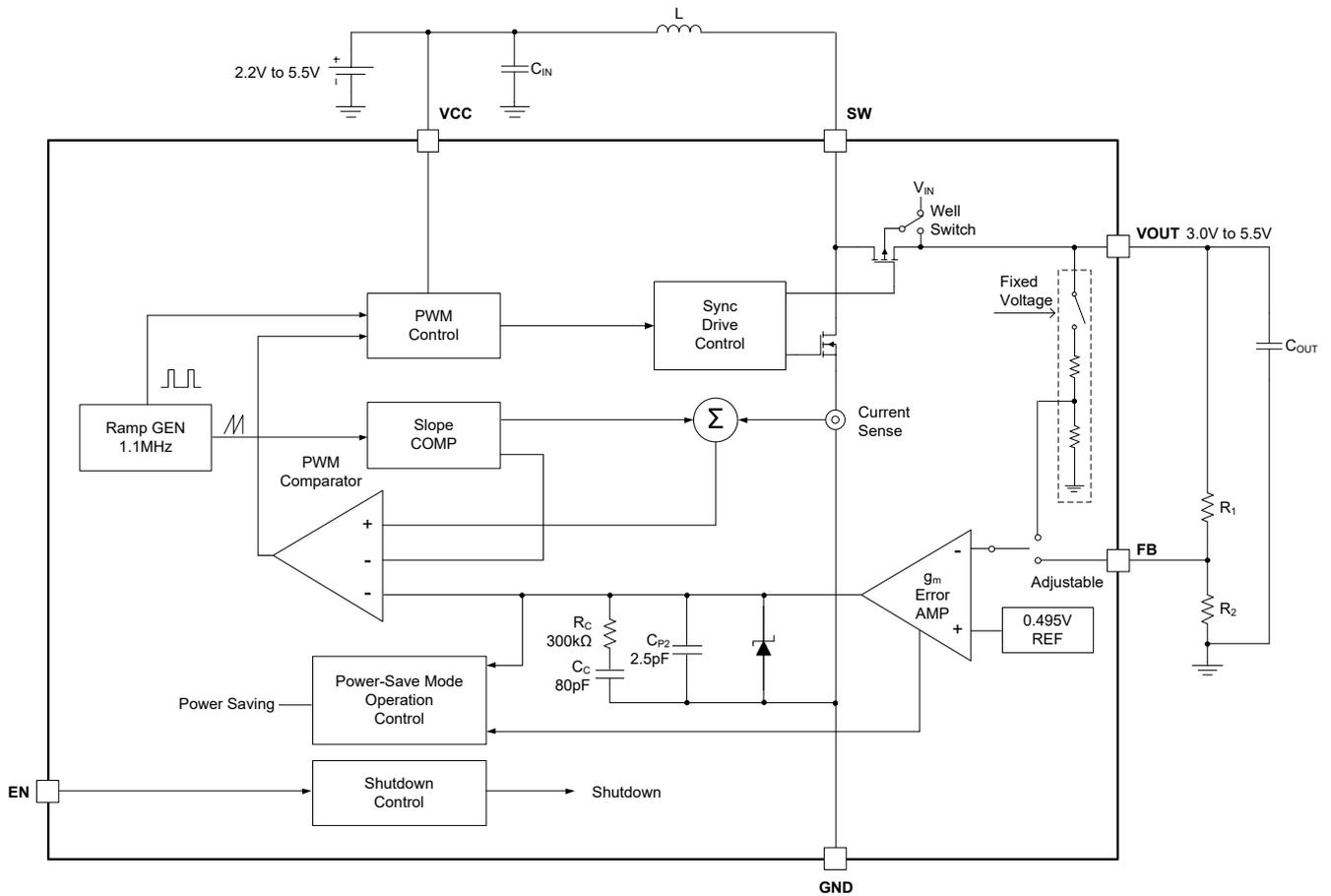
Figure 4. Block Diagram
