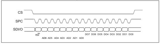
The SPI read command is performed with 16 clock pulses:
