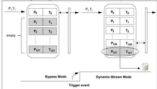
Figure 13. Bypass-to-Continuous (Dynamic-Stream) mode
