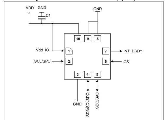
Figure 15. LPS27HHW electrical connections (top view)
