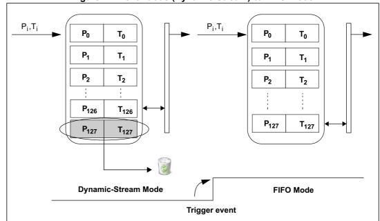
Figure 14. Continuous (Dynamic-Stream)-to-FIFO mode
