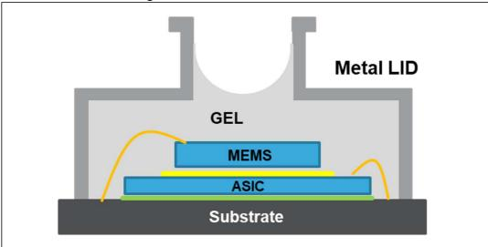
Figure 6. LPS27HHW internal structure
