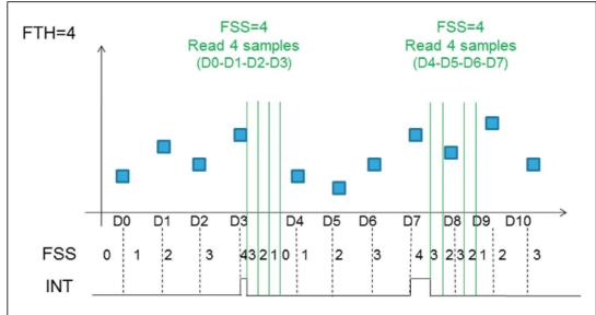
Figure 11. Continuous (Dynamic-Stream) mode
