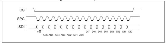
The SPI write command is performed with 16 clock pulses. The multiple byte write command is performed by adding blocks of 8 clock pulses to the previous one.
