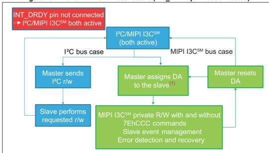
Figure 23. I<sup>2</sup>C and MIPI I3C<sup>SM</sup> both active (INT\_DRDY pin not connected)
