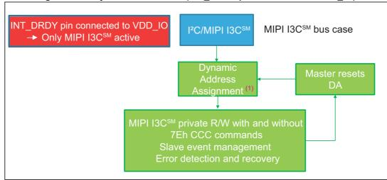
Figure 24. Only MIPI I3C<sup>SM</sup>active (INT\_DRDY pin connected to VDD\_IO)
