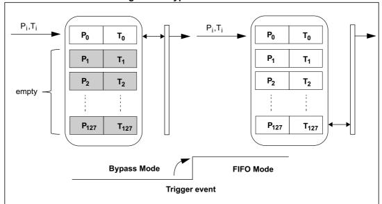
Figure 12. Bypass-to-FIFO mode
