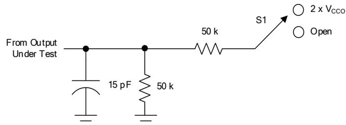
**Figure 3. Load Circuit For Enable/Disable Time Measurement**
