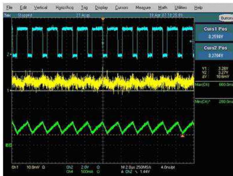
Figure 13. Ceramic 10 \mu F 0603 (X5R) (Good)
