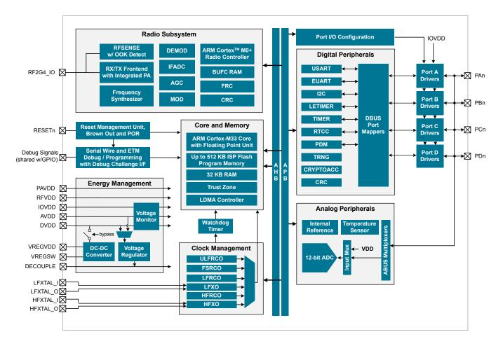
Figure 3.1. Detailed EFR32BG22 Block Diagram
