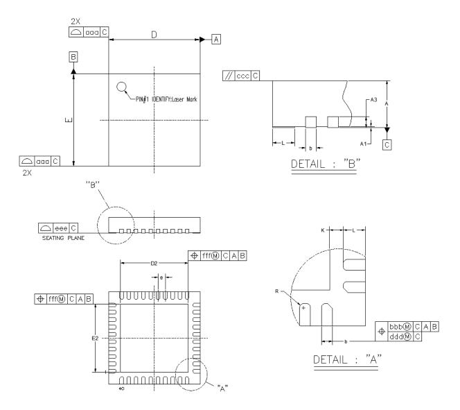
Figure 9.1. QFN40 Package Drawing
