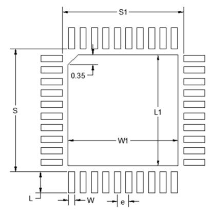
Figure 9.2. QFN40 PCB Land Pattern Drawing
