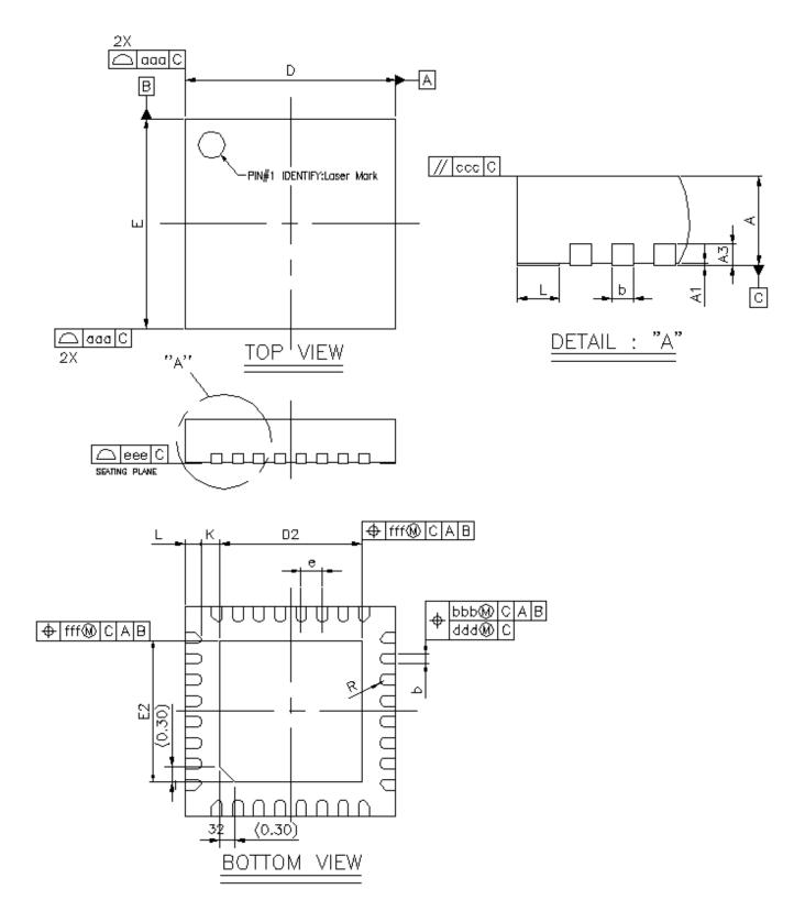
Figure 7.1. QFN32 Package Drawing
