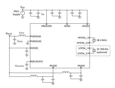
Figure 5.2. EFR32BG22 Typical Application Circuit: DCDC Configuration
