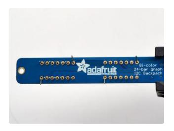
Turn over the PCB and bend oppositecorner pins of the modules out so that the modules are fixed in place against the PCB. Now is a good time to do a last check that you oriented the modules the right way!
