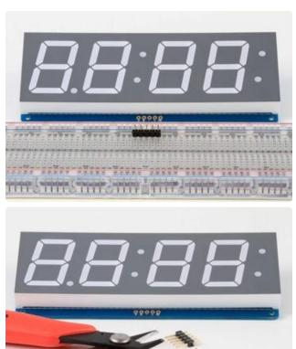
Cut the header strip to length if necessary and insert LONG pins down into the breadboard.
