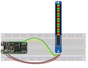
Microcontroller 3V to Bargraph VIN Microcontroller GND to Bargraph GND Microcontroller SCL to Bargraph SCL Microcontroller SDA to Bargraph SDA
