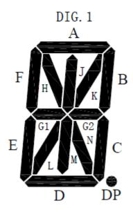
the 16 bit digit you pass in for raw image has this mapping:
