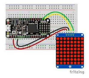
Microcontroller 3V to LED Matrix VIN Microcontroller GND to LED Matrix GND Microcontroller SCL to LED Matrix SCL Microcontroller SDA to LED Matrix SDA
