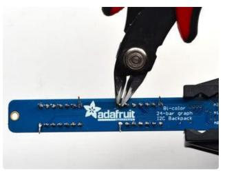
Once soldered, clip each pin. They're quite short and the pins are thicker than usual, so do this over/inside a trash bin so that the pins don't fly off and it you or your pets.
