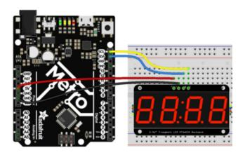
Backpack + (VCC) to microcontroller 5V (if using a board with 5V logic, otherwise use 3V for boards with 3V logic) (red wire)
