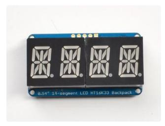
Remove the parts from packaging and place the LED matrices OVER the silkscreen side. DO NOT PUT THE DISPLAY ON UPSIDE DOWN OR IT WONT WORK!! Check the image below to make sure the 'decimal point' dots are on the bottom, matching the silkscreen.
