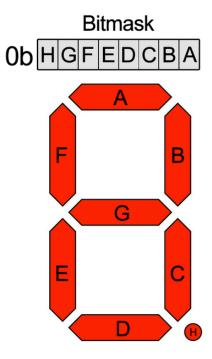
The bitmask is a single 8-bit number that can be passed in as a single Hexidecimal, Decimal, or binary number. This will use a couple different methods to display 8.8.EE:
