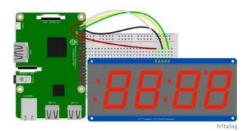
Raspberry Pi 3.3V to 7-Segment Display IO
