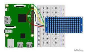
Raspberry Pi 3.3V to LED Matrix VIN Raspberry Pi GND to LED Matrix GND Raspberry Pi SCL to LED Matrix SCL Raspberry Pi SDA to LED Matrix SDA
