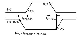
Figure 1. Switching Time Waveform Definitions
