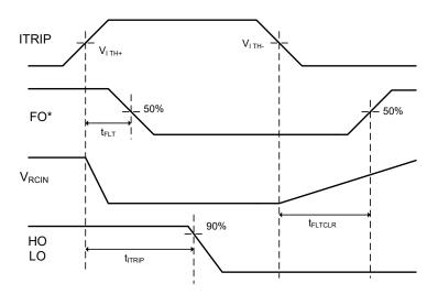
Figure 4. Overcurrent Timing Definitions
