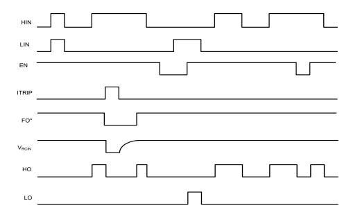
Figure 3. Input/Output Timing Diagram
