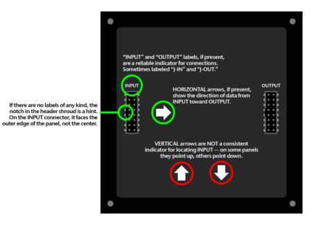
The arrangement of pins on the INPUT connector varies with matrix size and the batch in which it was produced...
