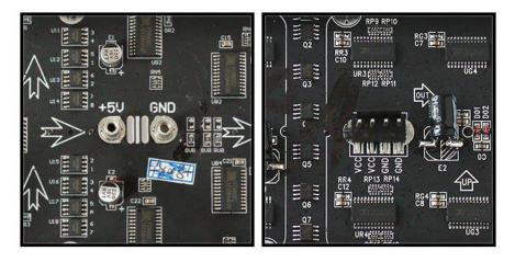
Two different types of power connectors have made an appearance:
