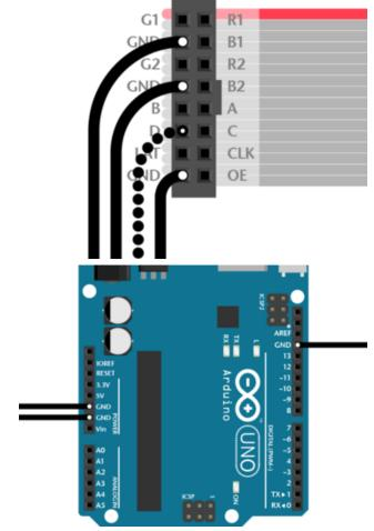
Current Arduino Uno form-factor boards have three ground pins (the third is next to pin 13). If you need additional ground connections — for a 32x16 matrix, or if using an older Arduino board with only 2 ground pins — a solderless breadboard is handy for linking all these pins.
