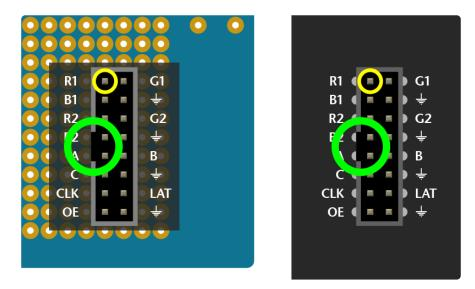
Wires are then soldered from the header to specific Arduino pins on the proto shield. Try to keep wire lengths reasonably short to avoid signal interference. Using color-coded wires helps a lot! If you don't have colored wires, that's okay, just pay close attention where everything goes. Our goal is a proto shield something like this:
