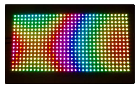
Of course, we wouldn't leave you with a datasheet and a "good luck!" We have a full wiring diagrams and working Arduino library code with examples from drawing pixels, lines, rectangles, circles and text. You'll get your color blasting within the hour! On most Arduino-compatible boards, you'll need 12 digital pins, and about 800 bytes of RAM to hold the 12-bit color image (double that for the 32x32 matrix, double again for smooth double-buffered animation).
