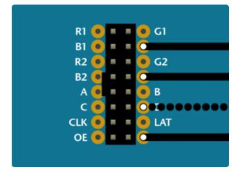
32x32 and 64x32 matrices require three ground connections. 32x16 matrices have four.
