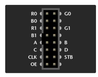
"Variant B" for 32x32 and 64x32 panels. The wiring is identical to Variant A above, only the labels are different.
