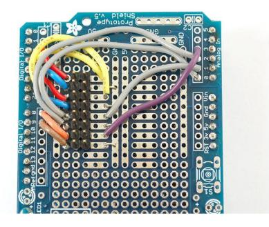
It's not necessary to install all the buttons and lights on the proto shield if you don't want — just the basic header pins are sufficient.
