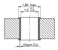
Drill hole specification for chemical surfaces (Ni/Au)
