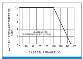
Fig.1- FORWARD CURRENT DERATING CURVE
