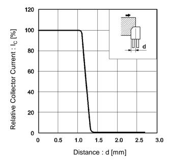
Fig.2 Relative Output Current vs.Distance (II)
