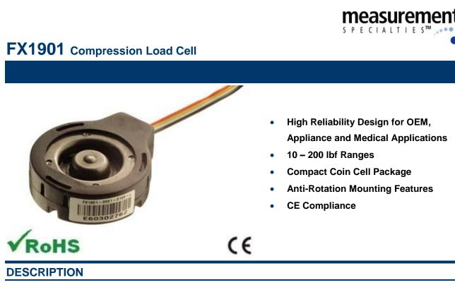
The FX1901 units are intended for OEM use in laboratory, hospital or consumer product applications, establishing a breakthrough price/performance value for compression load cells. The FX1901 is a 1% load cell device with full scale ranges of 10, 25, 50 or 100 and 200lbf compression. This new, low-cost technology enables force sensing in a whole new class of "smart" consumer and medical products.
