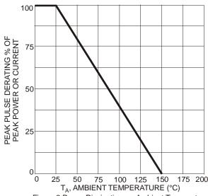
Figure 2 Power Dissipation vs. Ambient Temperature
