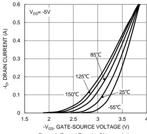
Figure 2. Typical Transfer Characteristic
