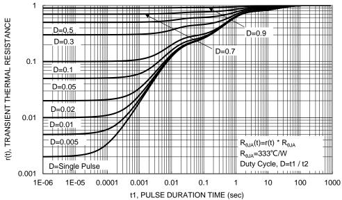
Figure 13. Transient Thermal Resistance
