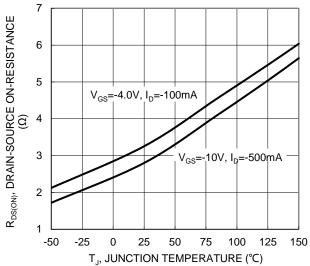
Figure 7. On-Resistance Variation with Junction
