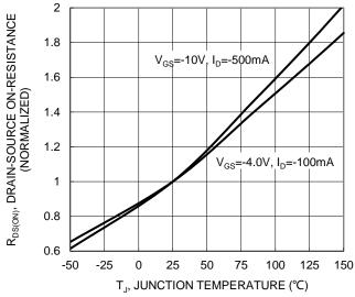
Figure 6. On-Resistance Variation with Junction Temperature
