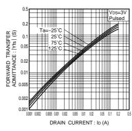
Fig.8 Forward transfer admittance vs. drain current
