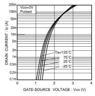
Fig.2 Typical transfer characteristics
