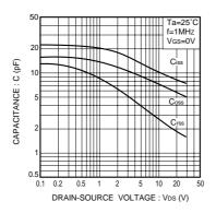
Fig.11 Typical capacitance vs. drain-source voltage
