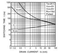
Fig.12 Switching characteristics (See Figures 13 and 14 for the measurment circuit and resultant waveforms)
