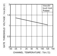
Fig.3 Gate threshold voltage vs. channel temperature
