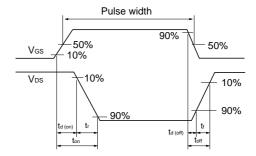
Fig.14 Switching time waveforms
