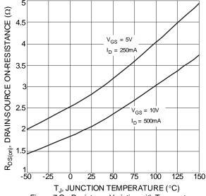
Figure 7 On-Resistance Variation with Temperature
