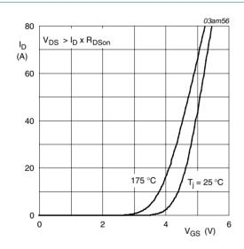
Transfer characteristics: drain current as a function of gate-source voltage; typical values
