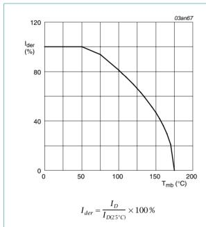
Normalized continuous drain current as a function of mounting base temperature
