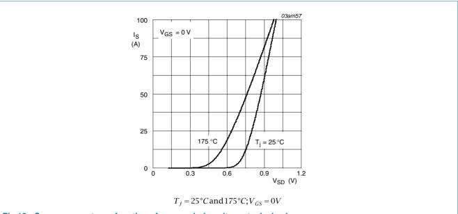
Fig 13. Source current as a function of source-drain voltage; typical values
