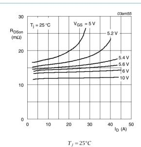
Drain-source on-state resistance as a function Fig 9. of drain current; typical values
