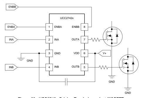
Figure 28. UCC2742x Driving Two Independent MOSFETs
