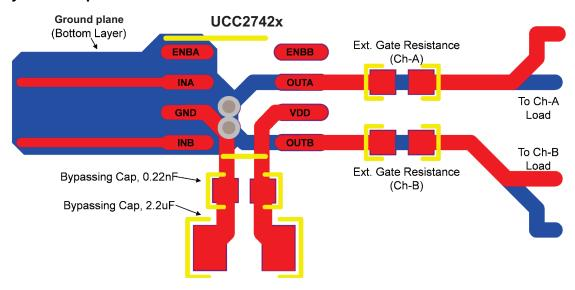
Figure 34. Recommended PCB Layout for UCC2742x
