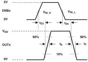
NOTE: The 10% and 90% thresholds depict the dynamics of the BiPolar output devices that dominate the power MOSFET transition through the Miller regions of operation.
