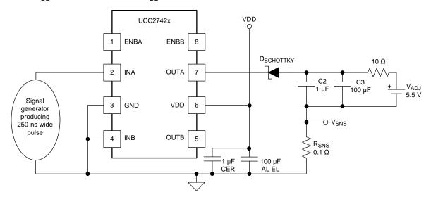
Figure 29. Current Sink Capability Test
