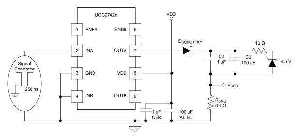
Figure 30. Current Source Capability Test
