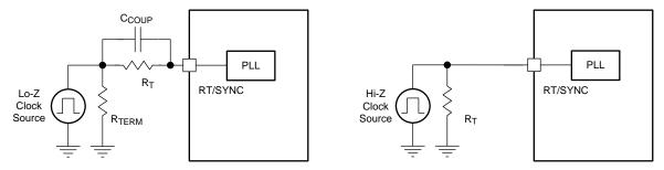
Figure 17. Synchronizing to an External Clock
