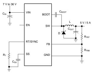
Figure 22. Application Circuit, 5V Output
