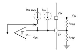
Figure 15. System UVLO By Enable Dividers
