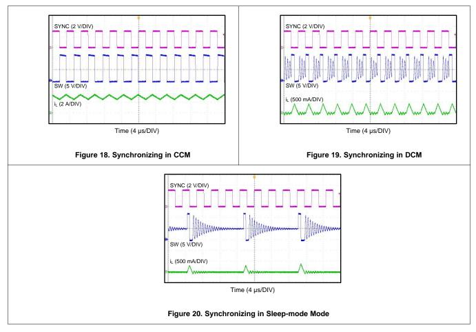
For spread spectrum option, the internal frequency dithering is disabled if the device is synchronized to an external clock.
