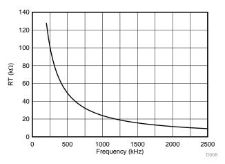
Figure 16. R<sub>T</sub> vs Frequency Curve
