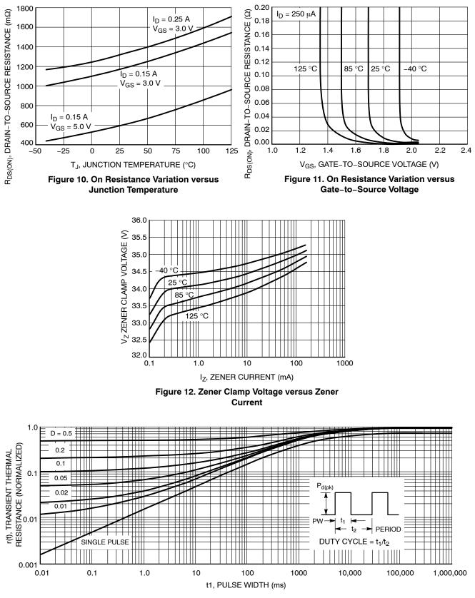
Figure 13. Transient Thermal Response for NUD3124LT1G
