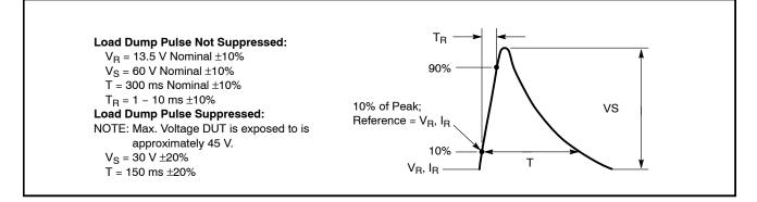
Figure 3. Load Dump Waveform Definition
