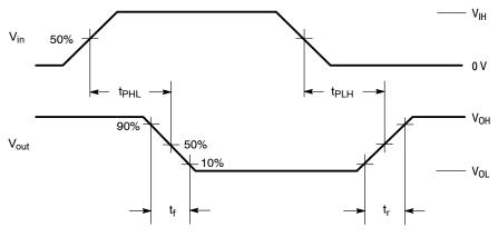
Figure 1. Switching Waveforms
