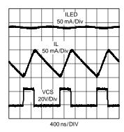
Figure 18. LED Ripple Current Reduction with a 1 µF Ripple Reduction Capacitor
