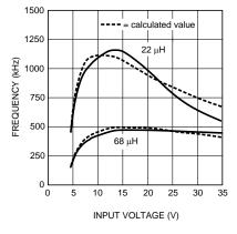
Figure 17. Frequency vs Input Voltage
