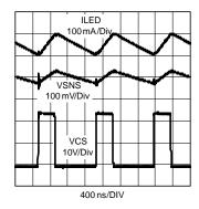
Figure 15. Hysteretic Switching Waveforms
