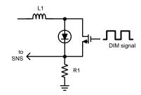
Figure 21. Parallel FET Dimming
