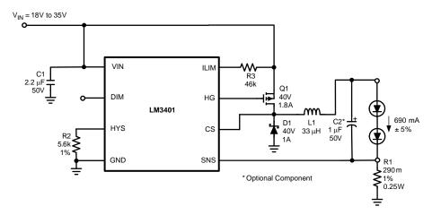
Figure 24. Example Circuit
