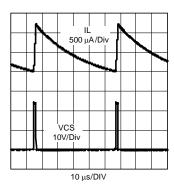
Figure 19. Typical Current Limit Operation
