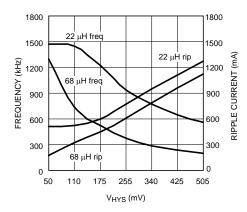
Figure 16. Switching Frequency and Ripple Current vs Hysteresis
