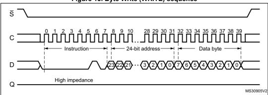
Figure 13. Byte Write (WRITE) sequence
