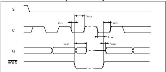
Figure 22. Serial output timing
