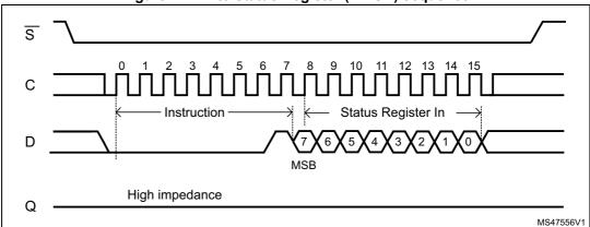
Figure 11. Write Status Register (WRSR) sequence
