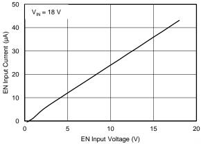
Figure 3. EN CURRENT vs EN VOLTAGE
