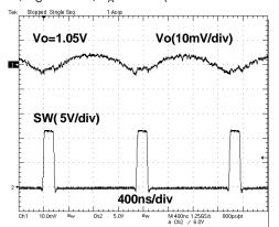
Figure 13. VOLTAGE RIPPLE AT OUTPUT (I<sub>O</sub> = 6 A)
