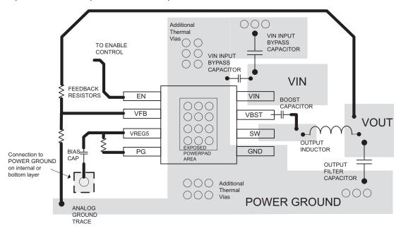
Figure 19. PCB Layout
