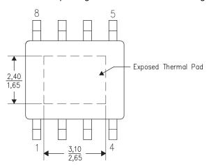
Figure 18. Thermal Pad Dimensions
