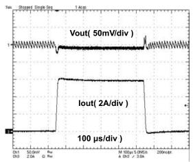
Figure 6. 1.05-V, LOAD TRANSIENT RESPONSE
