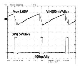
Figure 15. VOLTAGE RIPPLE AT INPUT ( $I_0 = 6 A$ )
