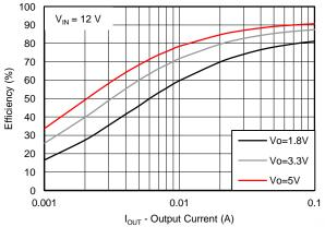
Figure 8. EFFICIENCY vs OUTPUT CURRENT
