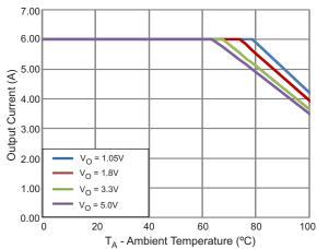
Figure 16. OUTPUT CURRENT vs AMBIENT TEMPERATURE
