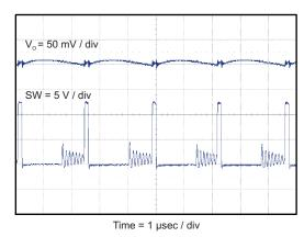
Figure 14. DCM VOLTAGE RIPPLE AT OUTPUT ( $I_0 = 30 \text{ mA}$ )
