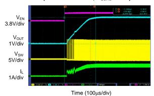
Enable Turn-off Characteristic (Resistance Load,  $R_{LOAD}$ =2.6 $\Omega$ )
