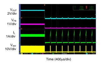
Short Circuit Recovery (R<sub>LOAD</sub>=2.6Ω)
