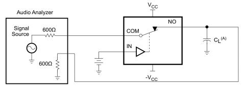
A.  $C_L$  includes probe and jig capacitance.
