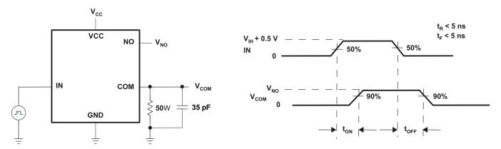
Figure 1. Switching Times
