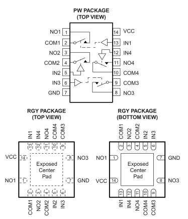
If the exposed center pad is used, it must be connected as a secondary ground or left electrically open.
