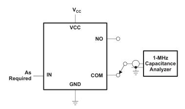
Figure 2. NO and COM Capacitance
