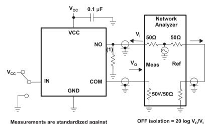
Measurements are standardized against short at socket terminals. OFF isolation is measured between COM and OFF terminals on each switch. Bandwidth is measured between COM and ON terminals on each switch. Signal direction through switch is reversed; worst values are recorded.
