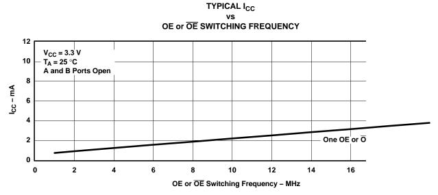
Figure 2. Typical I<sub>CC</sub> vs OE or OE Switching Frequency
