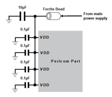
Recommended Power Supply Decoupling Capacitor Diagram
