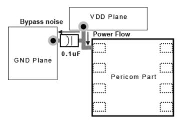
Decoupling Capacitor Placement Diagram
